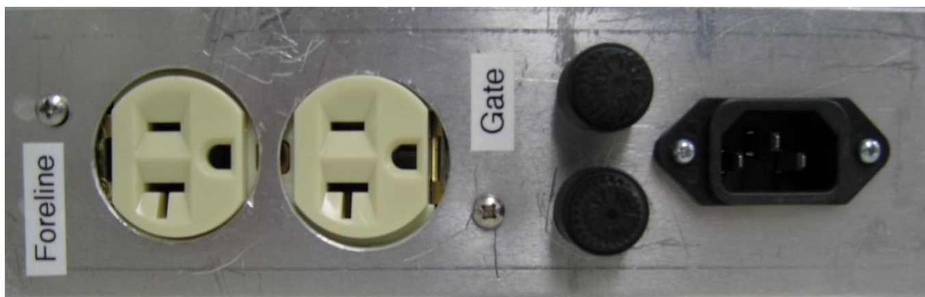
Back view of the vacuum fail-safe box.
