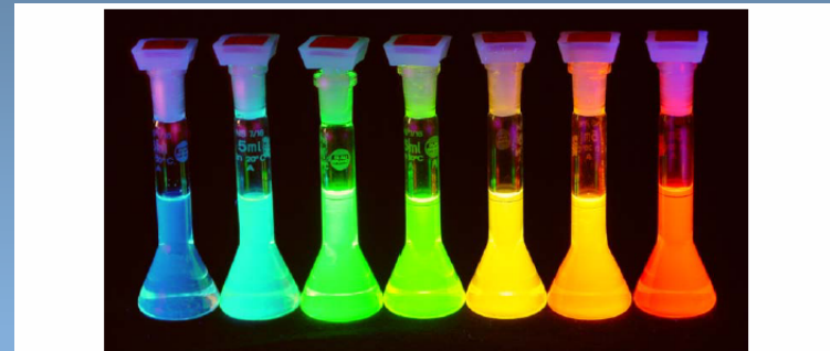
Figure 1.1. Size-dependent change of the photoluminescence color of colloidal solutions of CdSe nanocrystals passivated with a ZnS shell. The smallest (~1.7 nm) CdSe particles emit blue, the largest (~5 nm) – red.
