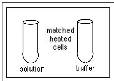
Heat is supplied at the same rate to two matched cells. The solution cell will generally absorb more heat than the buffer cell, causing a slight difference in temperature  $\Delta T$  between the two cells. A feedback loop monitoring  $\Delta T$  will supply a small amount of heat  $Q$  to the solution cell, so as to equalize the temperatures. The heat capacity  $C_p = Q/\Delta T$ .
