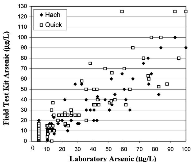
**FIGURE 2.** Quick Arsenic and Hach EZ field test kit and laboratory atomic fluorescence spectroscopy (AFS) arsenic measurements in the subgroup of 86 water samples with AFS arsenic levels at or below 100 µg/L. For some water sources with laboratory measurements  $\leq 100$  µg/L, the test kit measurements were above 100 µg/L.
