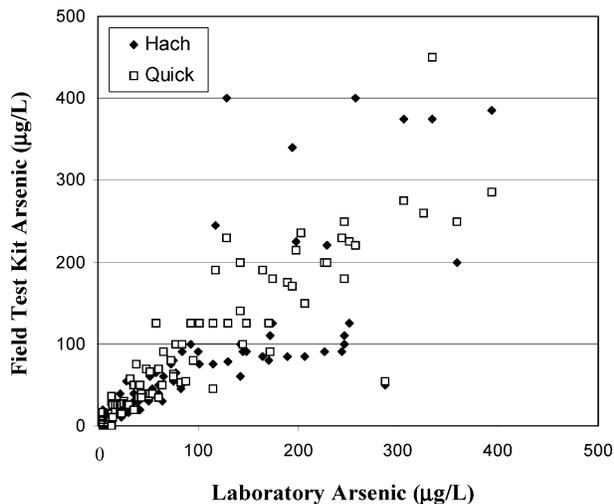
**FIGURE 1.** Arsenic measurements in all water samples with arsenic concentrations less than 500 µg/L ( $n = 118$ ) measured in the laboratory by atomic fluorescence spectroscopy (AFS) and the Quick Arsenic and Hach EZ field test kits.
