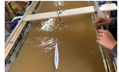
Figure 3. A 3D printed model of Bearneath the Sea is flume tested.
