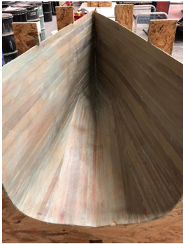
Figure 9: Full-scale mock-up of the end section of the canoe
