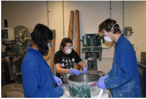
Figure 6. Testing new mix for workability and adding materials to improve quality
