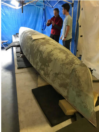
Figure 7. Demolded canoe exterior in need of patch mix
