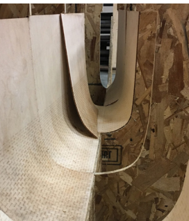
Figure 11: Panels with living hinges extending from the chine to the bottom of the canoe
