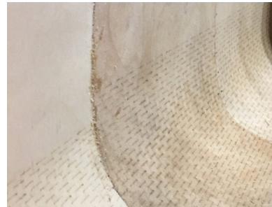
Figure 7: Panels with living hinges extending from the chine to the bottom of the canoe
