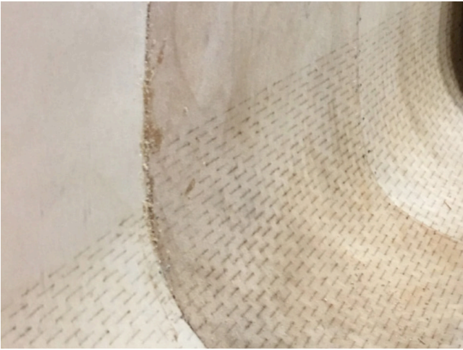
Figure 6. Panels with living hinges extending from the chine to bottom of the canoe
