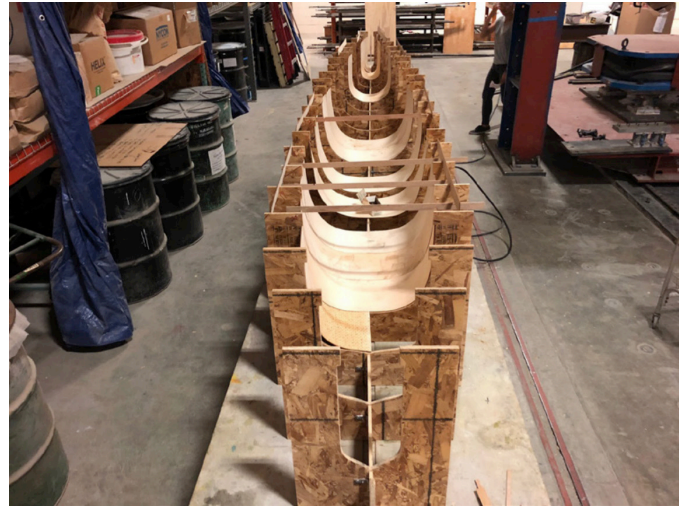
Figure 5. Interlocking skeleton with spacers for panel installation
