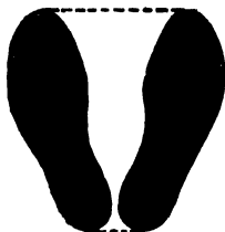
Fig. 16. When one stands, the perpendicular from the centre of gravity passes through the area bound by the soles of one's feet
