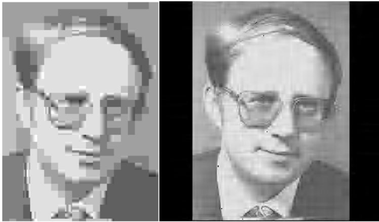
Figure 4: A comparison of images using 10:1 JPEG compression (left) and approximately 100:1 wavelet compression using the Daubechies-4 wavelet (right).
