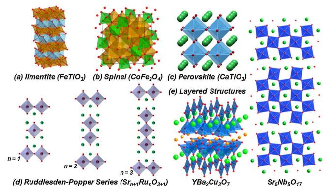
Fig. 2. Common ternary oxide crystal structures including (a) ilmentite, (b) spinel, (c) perovskite, and derivatives of the perovskite such as (d) the Ruddlesden–Popper series and (e) layered perovskites.
