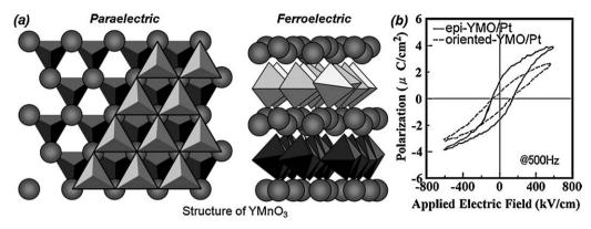
**Fig. 22.** YMnO<sub>3</sub>. (a) The crystal structure of YMnO<sub>3</sub> in the paraelectric and ferroelectric phases. The trigonal bipyramids depict MnO<sub>5</sub> polyhedra and the spheres represent Y ions. (Adapted from Ref. [289].) (b) *P*–*E* hysteresis of the epitaxial-YMO/Pt and the oriented-YMO/Pt. (Adapted from Ref. [315].)
