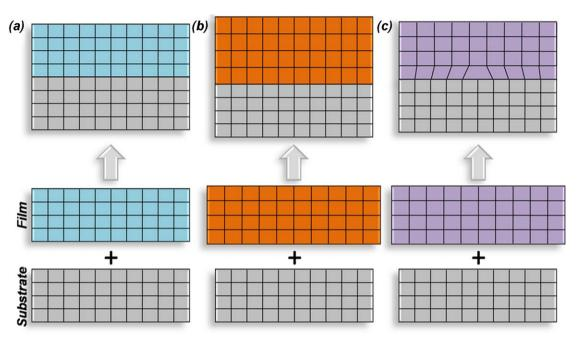
Fig. 5. Schematic illustration of (a) nearly perfectly lattice matched, (b) strained, and (c) relaxed heteroepitaxial film growth.
