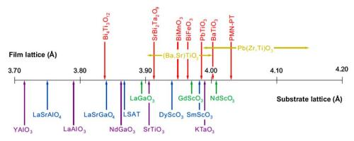
Fig. 10. Strain engineering. A number line showing the pseudotetragonal or pseudocubic *a*-axis lattice constants (in Å) of some ferroelectric perovskites of current interest (*above* the number line) and of some of the perovskite-related substrates that are available commercially (*below* the number line). (Adapted from Ref. [91].)
