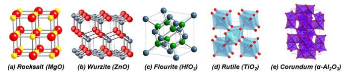
Fig. 1. Common binary oxide crystal structures including (a) rocksalt, (b) wurzite, (c) fluorite, (d) rutile, and (e) corundum.
