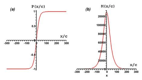
Fig. 26. Shape of ferroelectric polarization and magnetism across a domain wall in BiFeO<sub>3</sub>. (a) Ferroelectric polarization goes to zero at the center of the domain wall. (b) A net magnetization appears at the center of the domain wall even though the domains themselves do not possess a net moment. (Adapted from Refs. [377,378].)
