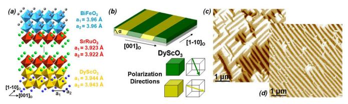
Fig. 14. Controlling ferroelectric domain structures. (a) Schematic of the BFO/SRO/DSO heterostructures and (b) domain structure of the BFO film as predicted by phase-field simulations. In-plane PFM images of the ferroelectric domain structure in BFO films showing (c) 4-polarization variants (left) and 2-polarization variants (right). (Adapted from Ref. [132].)
