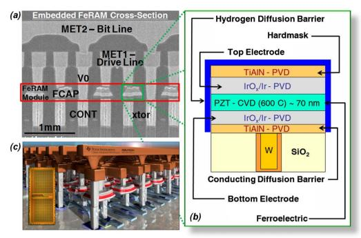
Fig. 17. Ferroelectric memories. (a) Cross-sectional scanning electron microscopy image of an actual ferroelectric memory device. (b) Schematic illustration of the FeRAM module showing all the layers needed for the creation of this device. (c) Artist's depiction of a FeRAM device, courtesy of Texas Instruments and Ramtron.
