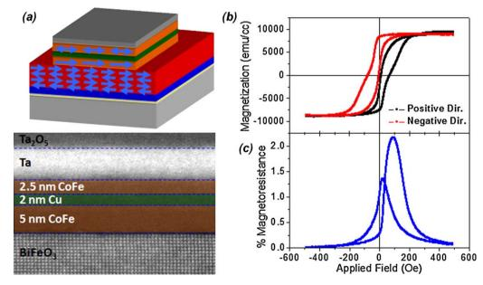
**Fig. 35.** Spin valve structures based on Co<sub>0.9</sub>Fe<sub>0.1</sub>/Cu/Co<sub>0.9</sub>Fe<sub>0.1</sub>/BiFeO<sub>3</sub> heterostructures. (a) Schematic illustration and scanning transmission electron microscopy image of the actual device. (b) Magnetic hysteresis loops of spin valve structures. (c) Current-in-plane magnetoresistance measurements. (Adapted from Ref. [437].)
