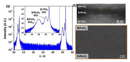
Fig. 25. Thin films of BiFeO<sub>3</sub>. (a) X-ray diffraction results from a fully epitaxial, single phase BFO/SRO/STO(0 0 1) heterostructure. (b) Low (top) and high (bottom) resolution transmission electron microscopy images of BFO/SRO/STO(0 0 1) heterostructure. (Adapted from Ref. [285].)
