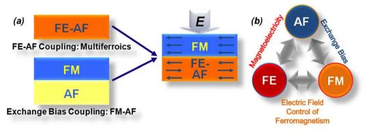
Fig. 34. Schematics illustrating the design algorithm for gaining electrical control of ferromagnetism. (a) By combining multiferroics together with traditional ferromagnets, we can create heterostructures that might have new functionalities. (b) These structure rely on two types of coupling – magnetoelectric and exchange bias – to gain electrical control of ferromagnetism. (Adapted from Ref. [285].)
