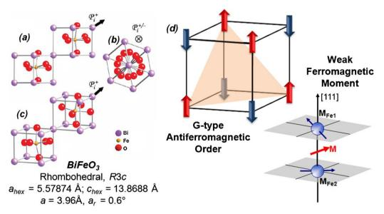
**Fig. 24.** BiFeO<sub>3</sub>. (a) Structure of BiFeO<sub>3</sub> shown looking (a) down the pseudocubic-[1 1 0], (b) down the pseudocubic-[1 1 1] polarization direction, and (c) a general threedimensional view of the structure. (d) The magnetic structure of BiFeO<sub>3</sub> is shown including G-type antiferromagnetic ordering and the formation of the weak ferromagnetic moment. (Adapted from Ref. [285].)
