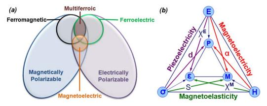
**Fig. 21.** Multiferroic and magnetoelectric materials. (a) Relationship between multiferroic and magnetoelectric materials. Illustrates the requirements to achieve both in a material. (Adapted from Ref. [286].) (b) Schematic illustrating different types of coupling present in materials. Much attention has been given to materials where electric and magnetic order is coupled. These materials are known as magnetoelectric materials. (Adapted from Ref. [285].)
