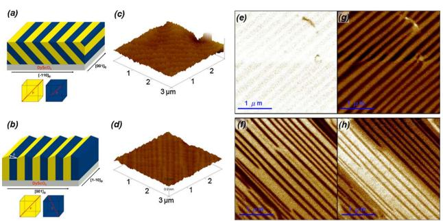
**Fig. 16.** Ordered arrays of ferroelectric domains and domain walls. (a) and (b) Schematics of equilibrium structure of an ordered array of 71° and 109° domain walls, respectively. (c) and (d) Surface topography as measured by AFM of 71° and 109° domain walls samples, respectively. Out-of-plane (e) and (f) as well as in-plane (g) and (h) PFM images for samples possessing ordered arrays of 71° and 109° domain walls. (Adapted from Ref. [135].)
