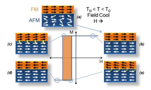
**Fig. 20.** Exchange bias. Schematic diagram illustrating the various stages of spin configuration in an exchange bias heterostructure being magnetically cycled. The diagrams show the spin configuration (a) above  $T_N$  under an applied magnetic field H, (b)–(e) below  $T_N$  at different applied magnetic fields. (Adapted from Ref. [266].)
