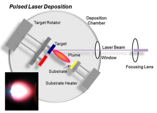
Fig. 6. Schematic of a standard pulsed laser deposition system. The inset picture shows an actual photograph of the plume.
