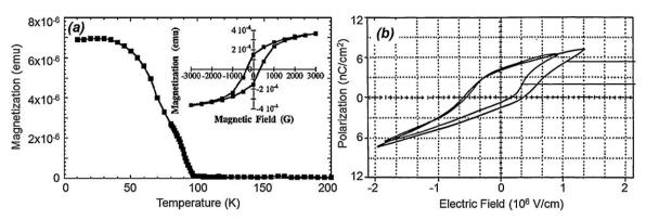
**Fig. 23.** BiMnO<sub>3</sub>. (a) Magnetization curve of a BiMnO<sub>3</sub> film cooled under no applied magnetic field. The inset shows the ferromagnetic hysteresis loop at 5 K. (Adapted from Ref. [327].) (b) *P*–*E* hysteresis loop of a thin film of BiMnO<sub>3</sub> on Si (1 0 0) above and below the ferromagnetic *T<sub>c</sub>*. (Adapted from Ref. [325].)
