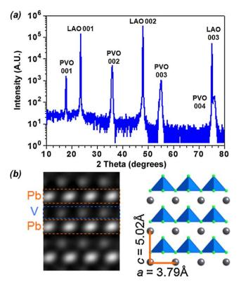
**Fig. 30.** Other multiferroics – PbVO<sub>3</sub>. (a) X-ray diffraction of a fully epitaxial PbVO<sub>3</sub>/ LaAlO<sub>3</sub> (0 0 1) thin film. (b) High resolution, cross-sectional transmission electron microscopy image of the PbVO<sub>3</sub> structure along with a schematic illustration of the large c/a lattice parameter distortion in this super tetragonal phase. (Adapted from Ref. [393].)
