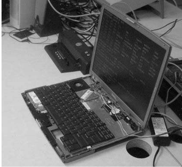
Figure 1.2: Dell notebook running Linux used for temperature measurements.
