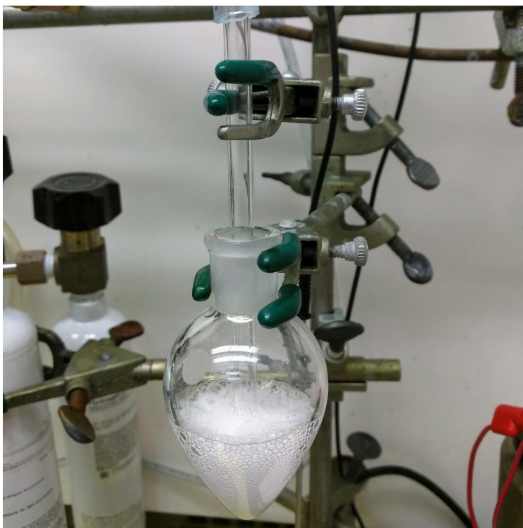
Figure B-7. Sulfuric acid sparge trap for ammonia capture and quantification by ^1\text{H} NMR.
