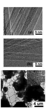
**Figure 1.** TEM image of (a)  $B_x C_y N_z$  nanotubes, (b) BN nanotubes, and (c) h-BN powder. Inset is the high-resolution TEM image.
