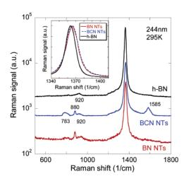
**Figure 2.** Raman spectra of BN and  $B_xC_yN_z$  nanotubes and bulk h-BN recorded at room temperature. Inset shows the main peak near 1366 cm<sup>-1</sup>.
