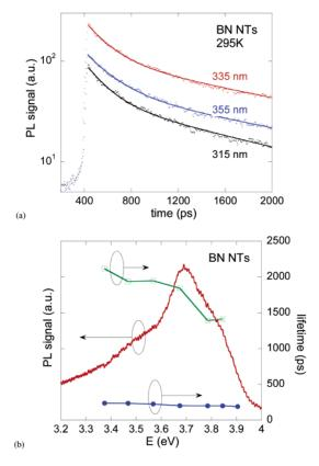
**Figure 4.** (a) Time-resolved photoluminescence of BN NTs. The wavelength window for each curve is 5 nm. The solid curves show the best fit using a double-exponential function. (b) Lifetimes obtained from the fitting with the double-exponential decay function.
