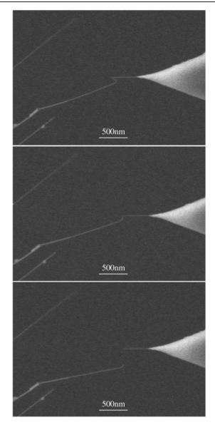
**Figure 2.** Top to bottom images show a sequence of the fabrication process of AFM carbon nanotube tips by the electron beam. The exposure of the multiwalled CNT to the electron beam produces the successive decapping of the CNT layers until it breaks in two. The final CNT tip is 300 nm.
