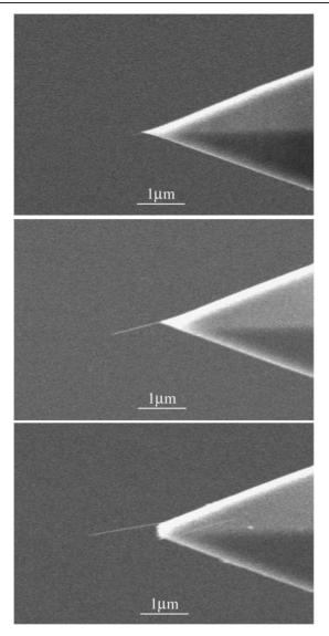
**Figure 3.** SEM images of several AFM carbon nanotube tips of different lengths (top to bottom) of 100, 1000 and 1500 nm.
