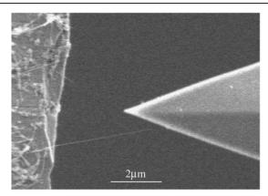
**Figure 1.** SEM image of an AFM silicon tip positioned closed to an isolated CNT aligned almost perpendicular to the metallic foil.
