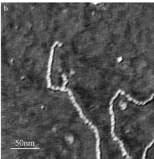
**Figure 5.** AFM images of double-stranded DNA deposited on mica. The images were acquired with CNT tips of lengths of (a) 300 nm and (b) 50 nm. Longer CNT tips produce ghost images while smaller CNT tips allow us to resolve periodic structures along the DNA molecule.
