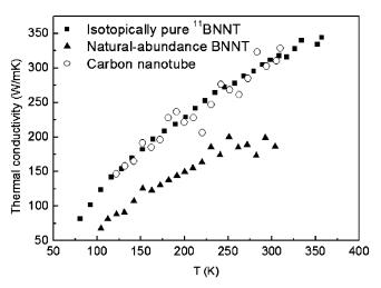
FIG. 2. The  $\kappa(T)$  of a carbon nanotube (open circles), a boron nitride nanotube (BNNT, solid triangles), and an isotopically pure boron nitride nanotube (solid squares) with similar outer diameters.
