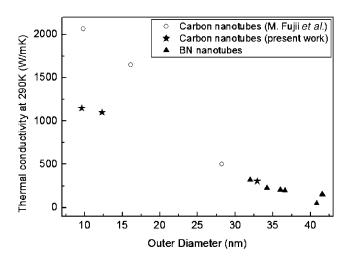
FIG. 3. The  $\kappa$ (290 K) vs outer diameter of various boron nitride nanotubes (solid triangles) and carbon nanotubes (solid stars). Data from Ref. [13] are also shown for comparison (open circles).
