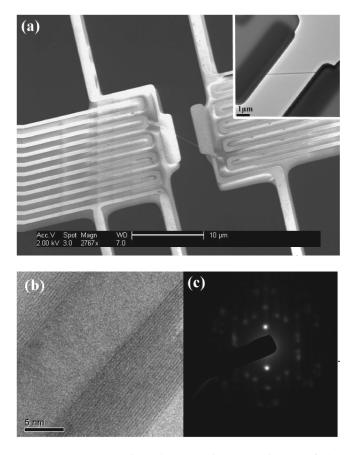
FIG. 1. (a) A scanning electron microscope image of the microfabricated test fixture with a boron nitride nanotube on it (scale bar = 10  $\mu$ m). The inset shows the corresponding transmission electron microscope image of the same device (scale bar = 1  $\mu$ m). (b) A high-resolution transmission electron microscope image of the boron nitride nanotube (scale bar = 5 nm). (c) The corresponding electron diffraction pattern of the boron nitride nanotube.
