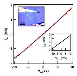
FIG. 2. (Color online) Source-drain current-voltage characteristic, with source-drain voltage  $V_{\rm sd}$  in the range of ±10 V, of the solder contacted graphene device shown in the inset, optical image (scale bar 10 μm, image contrast enhanced). Dashed line is linear fit to resistance 5.7 kΩ. Inset plot is low-bias *I-V* curve of same device, with a resistance of 6.0 kΩ. The back-gate voltage  $V_{\rm bg}$ =0 V.
