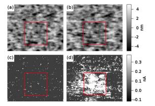
FIG. 2. (Color online) The  $1 \times 1 \ \mu m^2$  region outlined in red was scanned with a tip bias of 500 mV. Topographic maps of before (a) and after (b) reveal little change in the height profile, while the current maps before (c) and after (d) reveal a dramatic increase in conductivity.
