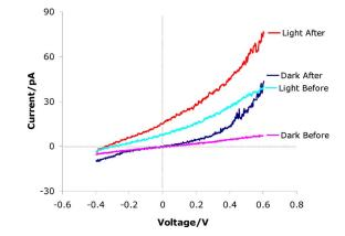
FIG. 4. (Color online) Current vs voltage response of the spot from Fig. 3 in dark and illuminated conditions before and after feature formation. Note that after the film has been locally current-injection treated, it exhibited much higher conductivity than before. The open circuit voltage increases from 0.29 to 0.33 V, and the short circuit current doubles from 7.6 pA before to 15 pA after.
