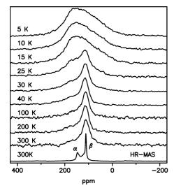
Figure 1. Static  $^{13}\text{C}$  NMR spectra of C<sub>60</sub> molecules encapsulated inside SWNTs at the indicated temperatures. Bottom spectrum: MAS  $^{13}\text{C}$  NMR showing the isotropic lines of the Cg<sub>0</sub> and Cg<sub>0</sub>.
