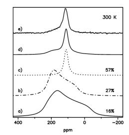
Figure 2. Simulated powder pattern line shape according to CSA tensor values described in the text for (a) SWNTs, (b) blocked  $C_{g_0}^{g}$ , (c) rotating  $C_{g_0}^{\beta}$ , and (d) the fit of the experimental spectrum (e) according to the indicated ratios.
