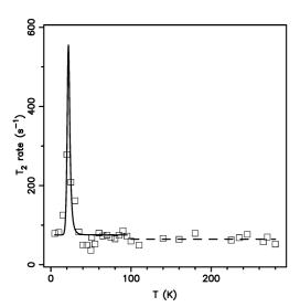
Figure 4. Spin-spin relaxation time  $T_2$  of  $C_{\beta_0}^{\beta_0}$  in peapods as a function of temperature. The peak occurs when autocorrelation rate  $\tau^{-1}$  is in the order of the line width (3 kHz at 4.7 T). Below 25 K, all the  $\alpha$  and  $\beta$  C<sub>60</sub> molecules are blocked.
