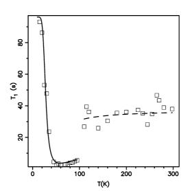
Figure 3. Spin–lattice relaxation time  $T_1$  of  $C_{00}^{\beta_0}$  in peapods as a function of temperature. The phase transition occurs at  $T_c = 100$  K. Note the abrupt change at  $T_c$  which occurs when  $C_{00}^{\beta_0}$  changes from continuous rotational diffusion (dashed line) to uniaxial rotation along the SWNT axis (solid line).
