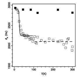
Figure 5. Second moment of the lines of the  $C_{60}^{\kappa}$  (solid square) and  $C_{60}^{\beta}$  (open square). Note the small increase (200 Hz) at  $T_c$  from the continuous rotational diffusion (dashed line) to uniaxial rotational motion along the axis of the SWNTs (solid line). Below 25 K, the  $C_{60}^{\beta}$  molecules are blocked, which is evidenced by an increase of  $\approx$ 800 Hz in  $\delta_{\nu}$ .
