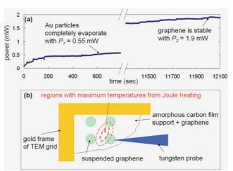
**Figure 3** (online colour at: www.pss-rapid.com) Joule heating power data and experimental geometry of the in situ experiment. (a) Joule heating power variation in time during the experiment. (b) Geometry of the in situ Joule heating experiment. Electrical current is flowing from the tungsten probe to the gold frame and inducing Joule heating on the suspended graphene and carbon film. Graphene regions between the gold frame and the tungsten probe reach the highest temperature in the sample.
