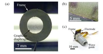
FIG. 2. Images of (a) 7 mm diameter graphene diaphragm suspended across annular support frame, (b) actuating electrodes, and (c) assembled speaker.
