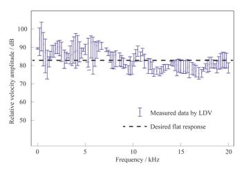
FIG. 4. Vibration velocity of graphene diaphragm in EDGS v.s. frequency, measured by LDV. Such a measurment is useful because it eliminates extrinsic effects (e.g., acoustic structural design, sound card, microphone response), and represents the "pure" response of the graphene diaphragm itself. Within the error limit of the LDV setup, the response curve appears to be quite flat, indicating that graphene serves as an ideal key component for loudspeakers.
