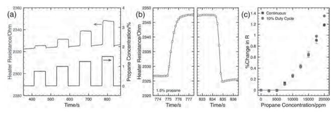
Figure 4. a) Pt-BN sensor resistance when exposed to varying propane concentrations showing stable, fast response. b) Sensor response (left) and recovery (right) shown in close up for 15 000 ppm propane exposure. c) Response of Pt-BN sensor versus propane concentration while heated to 500 °C continuously (squares) and for 100 ms every second (circles), which lowers the overall power consumption to only 1.5 mW.
