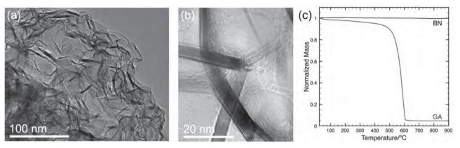
Figure 1. a) TEM of bare boron nitride aerogel. b) High resolution TEM of boron nitride aerogel showing highly crystalline, few layer BN. c) TGA of boron nitride aerogel<sup>[21]</sup> and graphene aerogel (GA), <sup>[37]</sup> showing improved thermal stability of the BN aerogel.
