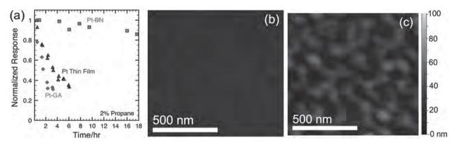
Figure 5. a) Normalized response to propane (2% or 20 000 ppm) versus time for Pt-BN sensors (squares), Pt-GA (diamonds), and an evaporated Pt thin film (triangles), showing the enhanced stability of Pt-BN sensor. AFM images of platinum thin film b) as evaporated (root mean square (RMS) roughness = 1.62 nm) and c) after 6 h of high temperature testing (RMS roughness = 12.18 nm) showing film agglomeration (Z-range of 100 nm in both images).
