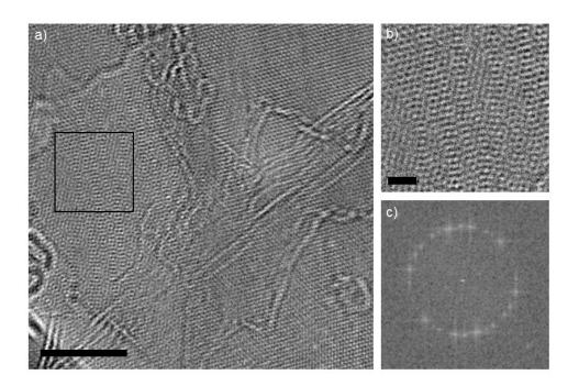
**Fig. S1** (a) TEM of a portion of BN aerogel and (b) a magnified region of the image in part a, showing a portion of BN sheets lying parallel to the imaging plane. (c) FFT of this region with at least 5 overlapping hexagonal spot patterns. Scale bars are (a) 5 nm and (b) 1 nm.
