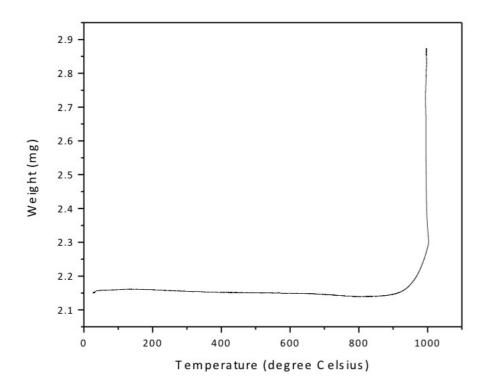
Fig. S6 TGA data for BN aerogel. The aerogel is stable up to 1000 °C.
