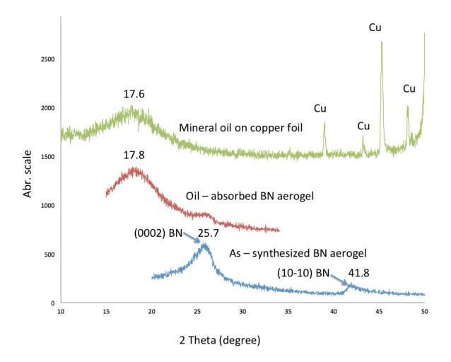
**Fig. S7** XRD patterns of as-synthesized BN aerogel, oil-absorbed BN aerogels and a mineral oil droplet on a copper foil. The broad peak approximately at 18 ° in oil-absorbed BN aerogel is apparently attributed to the mineral oil.
