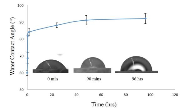
Fig. S4 Time – evolution of WCA of BN aerogel treated in UV – ozone plasma for 90 minutes.
