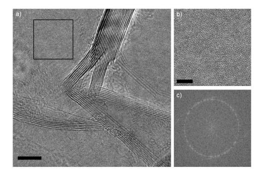
**Fig. S2** (a) TEM of a portion of BN aerogel and (b) a magnified region of the image in part a, showing a portion of BN sheets lying parallel to the imaging plane. (c) FFT of this region with at least 10 overlapping hexagonal spot patterns. Scale bars are (a) 5 nm and (b) 2 nm.
