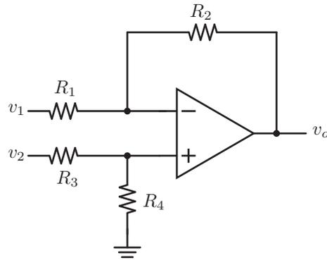
If we set  $v_2 = 0V$ , what is the gain from  $v_1$  to the output  $v_o$ ? (this is the inverting path)
