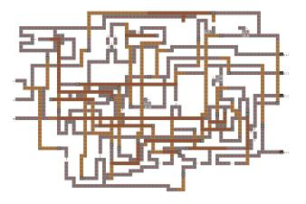
Figure 3: Extracted design of a four-bit counter.
