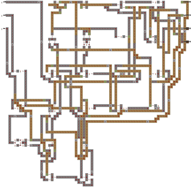
Figure 8. Completed PERSHING routing of a 4-bit counter based on the placement in Figure 7. Wires traveling on the stone layer (gray) are separate and do not intersect wires traveling on the wood layer (light brown). The two layers are connected by vias (not depicted).
