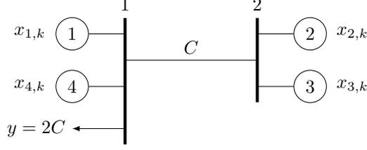
Figure 3: Example of a two-bus network in which the price of anarchy can be arbitrarily large.
