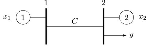
Figure 2: Example of a two-bus network in which a Nash equilibrium does not exist.
