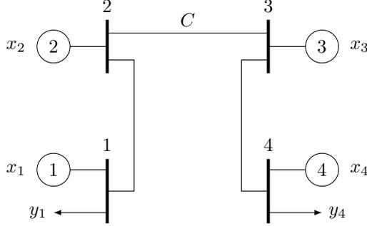
Figure 4: Example of a four-bus network which illustrates different equilibrium outcomes under different pricing mechanisms and offer formats.
