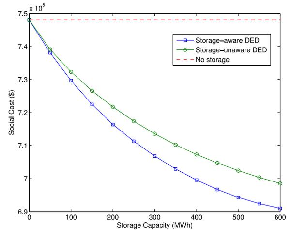
Fig. 5. Social cost versus storage capacity under three scenarios, when the flow limit is sufficiently large.
