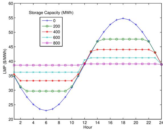
Fig. 7. LMP versus time under different storage capacities, when the flow limit is sufficiently large.
