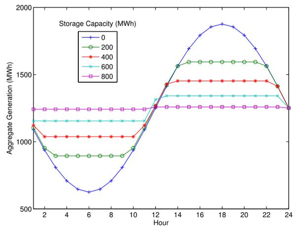
Fig. 6. Aggregate generation versus time under different storage capacities, when the flow limit is sufficiently large.
