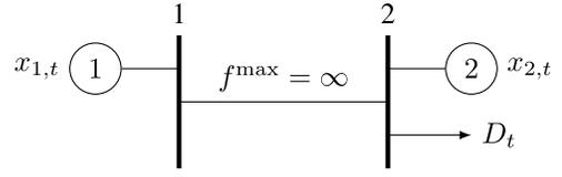
Fig. 2. Example of a two-bus, two-generator network.
