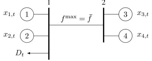
Fig. 3. Example of a two-bus, four-generator network.
