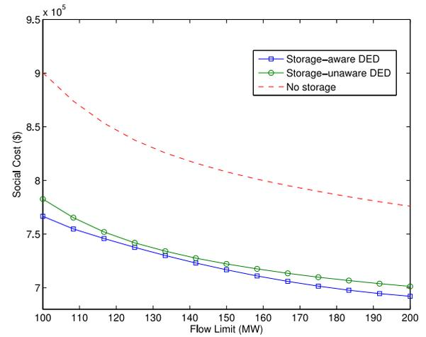
Fig. 4. Social cost versus flow limit under three scenarios, when the storage capacity is sufficiently large.
