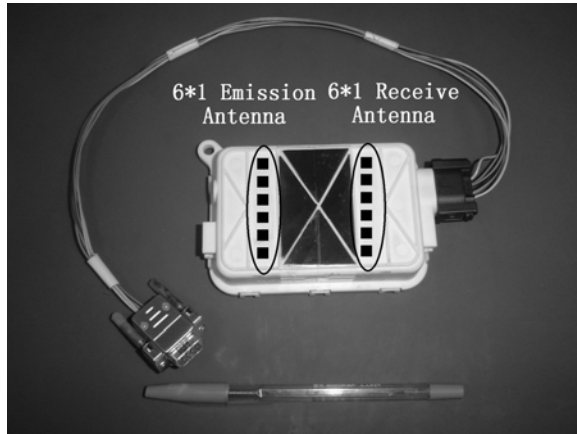
Fig. 2. HRR microwave radar, in contrast with a ball pen.
