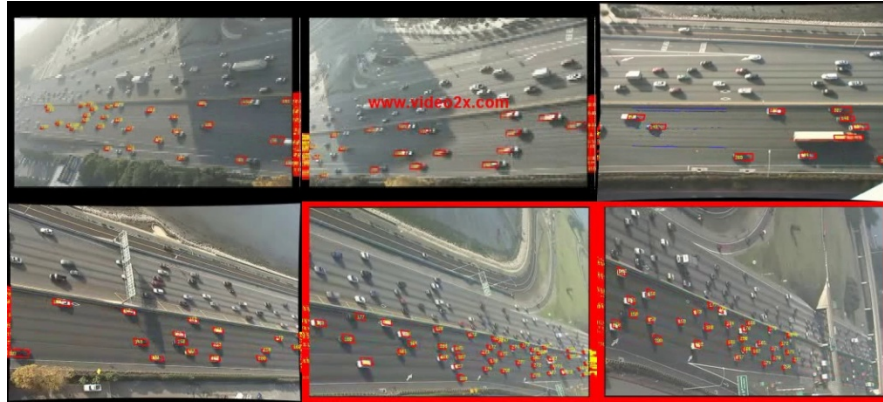
FIGURE 1 Original pictures of traffic observation in the NGSIM project. Red rectangles belong to tracing software (5).
